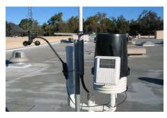
In December 2008 the GSA Grounds Department installed a weather station at the GSA Service Building located on the Government Center Campus. The wireless system sends valuable information to our Central Irrigation Computer. The weather station provides
